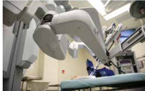
With sophisticated cameras and robotic arms operated by physicians, the da Vinci® surgical robot provides doctors easier access to operate, but without the need for open incisions.
